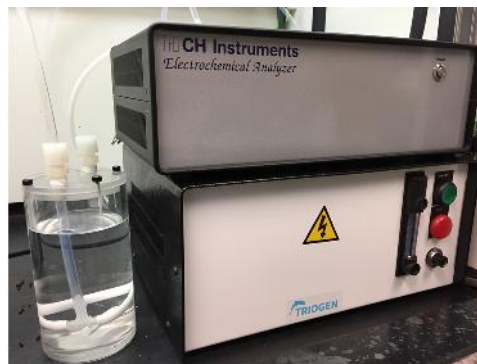
Figure 3. Ozonation/Electrolysis System Used for Treatment Studies
